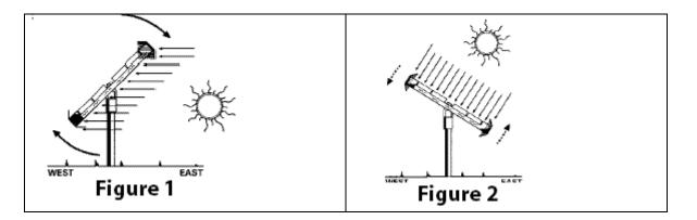
The movement of the liquid is controlled by the aluminum shadow plates mounted on the outside of each canister. When one canister is exposed to the sun more than the other, its vapor pressure increases which forces liquid freon to the cooler shaded side.
